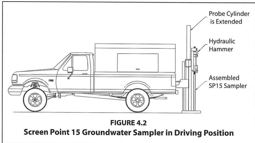
4. Repeat Step 3 until the desired sampling interval is reached. Approximately 12 inches (305 mm) of the last probe rod must extend above the ground surface to allow attachment of the puller assembly. A 12-inch (305 mm) rod may be added if the tool string is over-driven.
