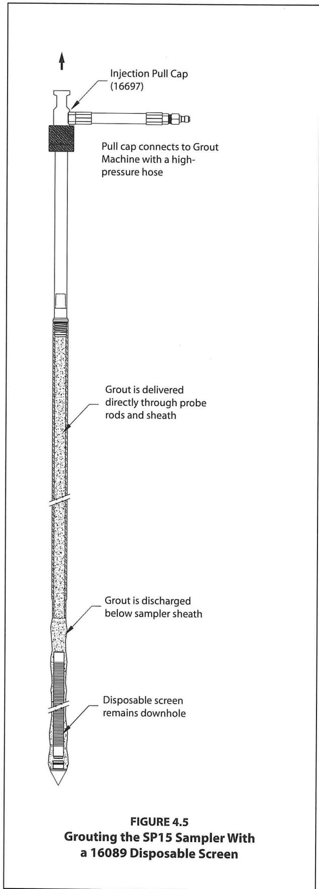
3. Place a mark on the extension rod even with the top of the probe rod. Apply downward pressure on the extension rods and push the grout plug out of the screen. The mark placed on the extension rod should now be below the top of the probe rod. Remove all extension rods.
